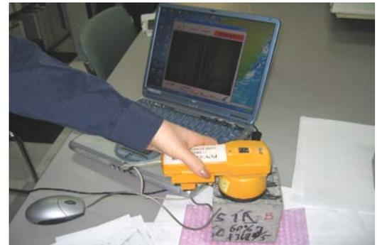
Fig. 3 Apparatus for measuring scratch width
