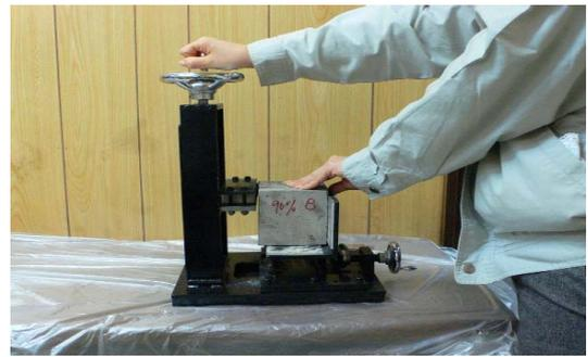
Fig. 2 Apparatus for scratch test
